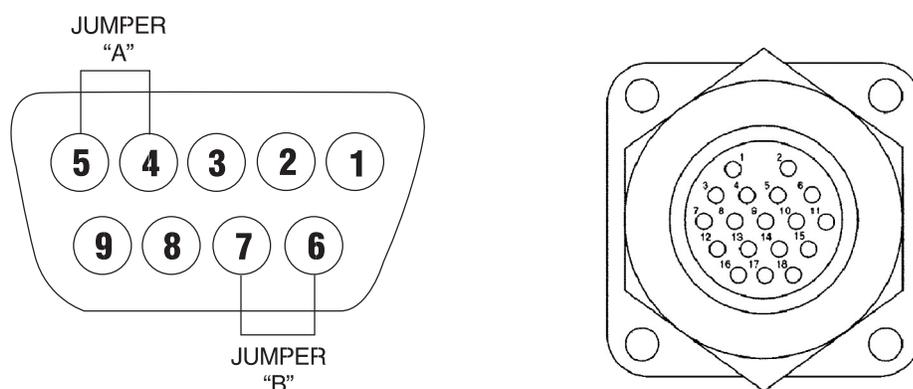
**Note:** Jumpers “A” and “B” are optional. See *page 3-3 External Inputs* for correct usage.
